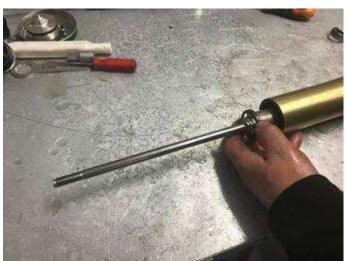
8. Discard the compression adjuster and copper washer plus all of the open cartridge assembly.
