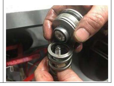
5. Remove the fork spring and invert the fork leg to drain the oil from the leg, try and put one finger over the top of the piston rod to prevent the 5 mm diameter aluminium rebound needle from falling out when the fork leg is upside down. It is useful to stroke the piston rod up and down slowly to help remove the oil from inside the fork leg.
