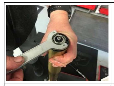
3. Invert complete fork leg (placing a soft rag on the floor to prevent damage to the fork preload cap) and proceed to start filling with 5W oil through the axle clamp hole. Ensure that the volume of oil being filled is recorded, as there is a total volume needed for each fork leg (450ml total per leg), and it is generally not possible to fill the full amount from the bottom.
