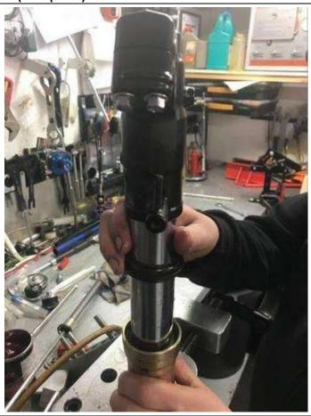
2. Remove the wire clip, using a small flat screwdriver and then warm the outer section of the aluminium tube, next to the fork seal with a hot air gun, this will expand the aluminium slightly to make removal of the inner fork leg easier.
