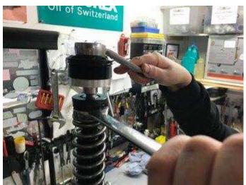
14. Check that the whole assembly looks correct, and in line, slide the fork outer up to meet the fork cap, start tightening by hand, until resistance can be felt, then use the special pin tool provided, to tighten the cap into the tube as tight as possible by hand.
