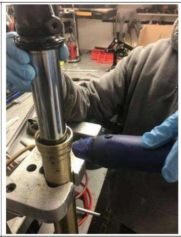
3. Using a sliding action, remove inner fork stanchion from outer leg by repeatedly sliding backwards and forwards until it comes out completely.
