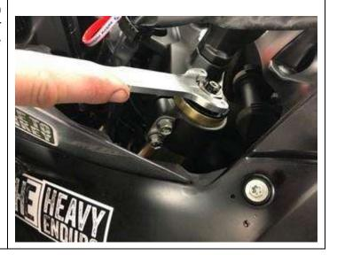
3. Reattach the front fender with the 2 screws on the lower fork leg, we recommend that the outside steel screw of the fender be replaced with one of our nylon screws, so that in the event of the fork hitting a rock or tree stump, the nylon screw will break rather than the steel screw, forcing the cast lug on the lower fork leg to snap off.
