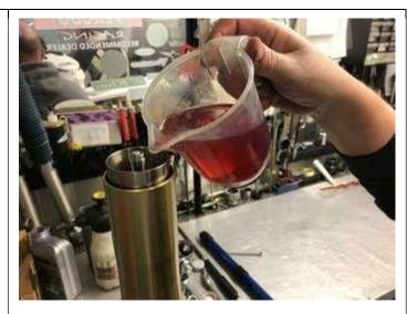
10. Check the oil height (air gap), which is 120mm from the top of the inner fork tube (with outer tube level with inner) if too much oil is put in, and the fork has to be tipped over to pour out the excess oil, it will be necessary to move the fork up and down a few times to make sure the fork is fully bled of air, before repeating the operation to get the oil height correct. Recommeded 120mm oil level is set without spring and compressed forkleg and damper rod fully compressed.
