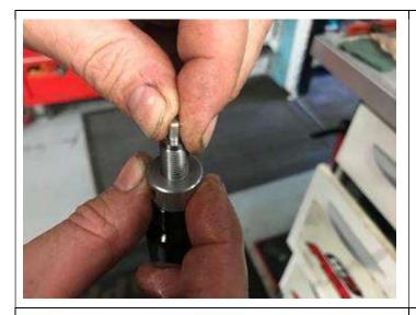
12. The preload caps for the fork come complete with three plastic washers per cap, these can be mixed in any combination if they have the same thickness for each fork cap.
