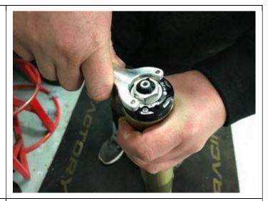
16. Check the axle clamp bolt is fully tightened (40Nm) by holding fork leg lower in a vice (with soft jaws) and clean the forks fully. If the bolt keeps turning because the cartridge is spinning inside the fork leg, then try to use an impact wrench (on low setting) to tighten it before attempting using a torque wrench again.
