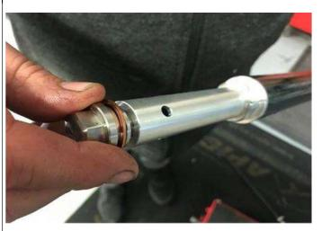
2. Insert the new open cartridge (with fork cap attached but no spring fitted) into the fork leg enough until it contacts the bottom of the lower stanchion and tighten the screw cap on top of the fork leg - hand tight only using tool supplied.
