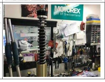
15. Push the fork leg up and down by hand, with the bottom of the fork leg on the floor, it should move slowly and without any harshness.
