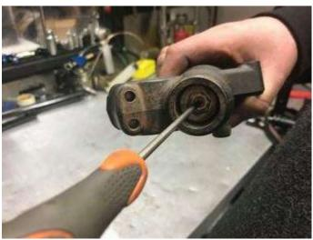
2. Invert the fork leg and hold in a suitable clamp then using a 14 mm hexagon bit, undo the compression adjuster at about half a turn to break the seal.
