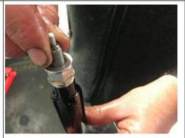
9. Do not allow the outer fork tube to go more than 10mm past the top of the chrome inner tube (as shown) or there is a risk that the top DU bush can pop out of the recess and lock the forks. To help expel any remaining air from the cartridge, pull the fork out up to full extension and place palm of hand over open end, and then compress fork, the increased air pressure will push the oil into the cartridge.
