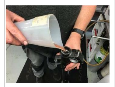
4. Fill with small amounts at a time, no higher than the bottom of the threaded hole in the cartridge, lift up the axle 100mm approx. then compress the fork whilst covering the opening with the palm of the hand. This causes air pressure to force the oil into the cartridge.
