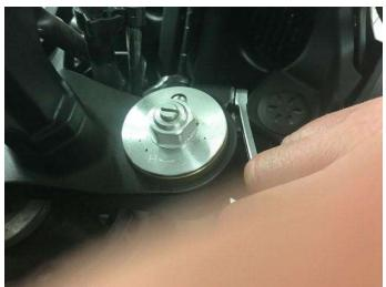
7. Using a 19 mm spanner, undo the fork cap slightly.
