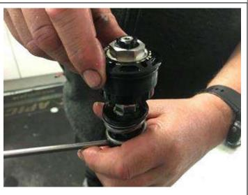
13. Place the required plastic washers onto the top of the spring, and then screw on the fork cap by hand until resistance is felt. Tighten fully using a 22 mm spanner on the fork cap and a 17 mm spanner on the aluminium nut.
