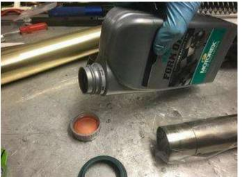
7. Lubricate the inner of the dust seal and slide it onto the fork leg, ensure it goes on the correct way as per the photographs. Next slide on the wire clip, and then lubricate the fork seal, and slide it over the end of the fork gently, so as not to damage the seal lip.
