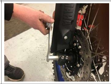
5. Tighten axle fully by hand.
