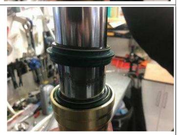
11. Lastly, push in the dust seal, and wipe any excess oil from the whole assembly.
