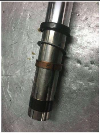
4. Prize off the top bush by opening the gap and sliding it off the top of the fork leg, the next bush slides straight off, along with the steel washer, then the oil seal, metal clip and dust cover.
