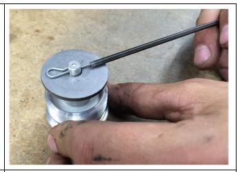
12. Fit locking washer clip (supplied with kit) on to centre shaft, making sure the tags point slightly up, then using a tube or socket tap them down until it seats with the steel washer
