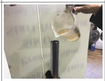
9. Work fork up and down a few times to free any trapped air bubbles. Then drop in damper piston assembly, threaded end first, into fork leg. Next drop in spacer tube, stepped end first, above piston assembly. Pour in the remainder of the 10W fork oil and work fork slowly up and down to remove trapped air. It can help to extend the fork fully, then cover the open top of the fork tube with the palm of the hand, and push down, this will pressurize the fork and help remove trapped air.
