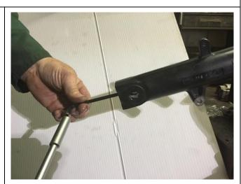
4. Remove fork cap by holding upper fork tube and undoing cap. Compress fork slightly, remove plastic spacer and pull out fork spring, DISCARD BOTH SPACER & SPRING. Remove fork leg from vice and invert slightly to tip out damper rod and short top-out spring. Pump fork slowly to remove all oil from chamber.
