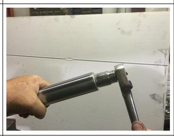
15. Fully tighten Allen screw in bottom of fork leg, then remove leg from vice and work up and down to check movement and damping.
