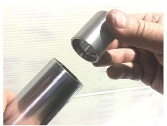
10. Once satisfied that all air is removed, drop new plastic liner into fork tube, as shown in picture. Then insert fork spring into extended leg, the spring should seat over the collar of the plastic liner, as a centering guide for the spring.
