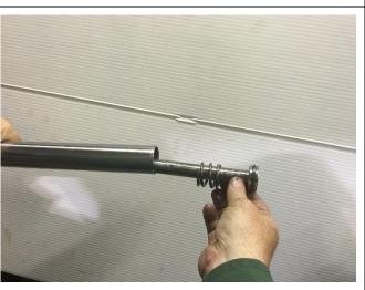
5. Remove split seal from OEM damper rod, and fit to new damper rod. Fit OEM top-out spring onto shaft of new damper rod, and slide into fork. Hold lower fork in vice, with soft jaws, or with cloth protection, at about 45 degrees angle.
