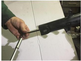
8. Remove fork from vice and remove fork spring, slide fork in and out, to check free movement pour in 150ml of 10W Fork Oil
