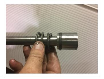
6. Put new fork spring into fork and apply pressure to damper rod, to ensure alignment of damper rod in bottom of fork leg, it can help to insert a small screwdriver up through the hole in the bottom of the leg which should go into the threaded hole in the bottom of the damper rod.
