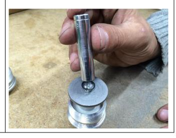
13. Holding fork tube by hand, or if in a vice use soft jaws and hold the tube near the top where the seals do not run. If the spring and damper rod components are seated correctly then with the fork at full extension the spring should extend through the top of the tube by several mm. Insert existing Pre Load Adjuster into fork tube a few turns by hand.
