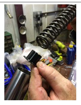
11. Remove existing R Clip from OEM Pre Load Cap on underside, do not remove steel washer.
