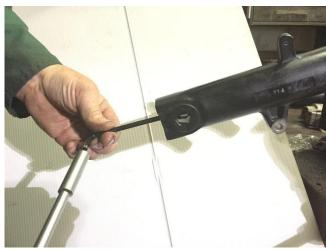
16. Clean off all oil from outside of fork with cloth and refit into triple clamps.
