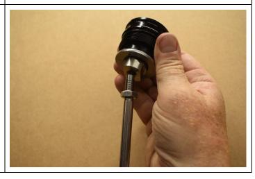
16. Holding the rod, tighten the new cap down fully until it bottoms internally, there will be a small gap between the underside of the cap and the lock nut. Using the pin socket and 30 mm spanner, along with14mm spanner on the lock nut, tighten both together.
