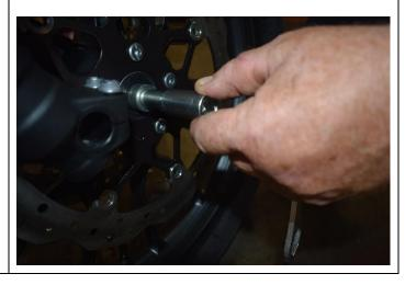
32. Remove both caliper bolts and slide caliper into position on the disks, it may be useful to push back the brake pads before doing this to give more space when inserting them.
