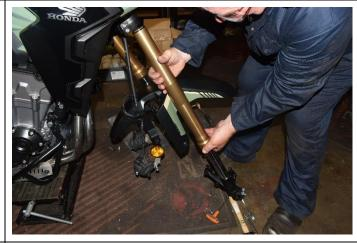
11. Clamp leg in a special fork vice or a vice with soft jaws. using a 41 mm spanner, undo the fork cap completely. Compress fork to expose cap and rod.
