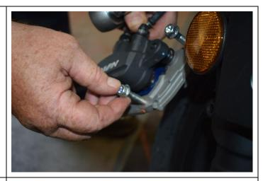
33. Apply Red (Strong) Loctite™ to the threads of both caliper bolts and insert into the caliper, tighten by hand using 12 mm socket then torque fully to 36 nm
