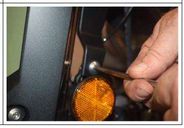
29. When attaching front lower screw ensure that the rubber "top Hat" liner on inside of the fender, above the screw, is aligned with the metal pin on the fork leg casting.
