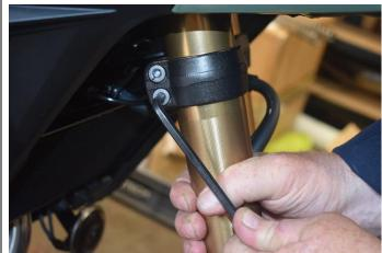
Using a 41mm octagonal spanner, undo the righthand fork cap about one turn. Whilst holding the lower fork leg undo both lower triple pinch bolts and remove whole leg.
