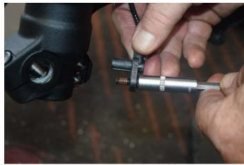
28. Re- attach both fender screws into each fork leg using a 5mm Allen Key. Do not tighten fully.
