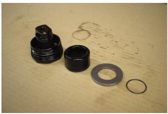
14. Take the new Rally Raid fork cap, insert the rubber sleeve, then the metal washer and finally the wire clip, making sure the clip is seated in the groove.
