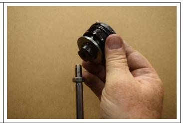
13. Invert the fork cap and remove the wire clip using a small flat screwdriver, remove the steel washer from the fork cap and then lever out the rubber sleeve, again using a flat screwdriver.
