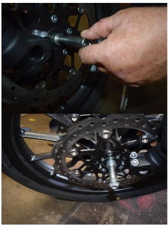
Using 12mm socket, remove both left-hand caliper bolts, detach caliper, replacing bolts in caliper. Repeat for opposite leg.
