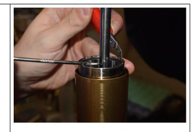
19. Withdraw top out assembly, you may need to tap the underside of the fork cap to dislodge the steel ring that is inside the fork tube. You will not be using the top out assembly, but we advise you keep safe, should you need to return the forks to standard.
