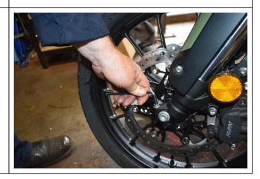
Undo both right hand fork pinch bolts using 6mm Allen Key.
