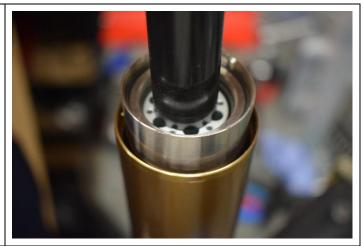
22. Remove fork leg from vice, extend fork and tighten fork cap by hand, then tighten further using pin socket and 13 mm spanner.
