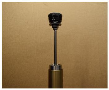
12. Using a 41 mm spanner and a 14mm spanner, undo the locknut that is below the fork cap, from the shaft. Remove fork cap.
