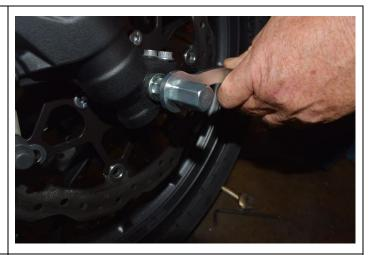
3. Replace spindle through wheel and re-insert bolt from opposite side to prevent loss of spacers.
