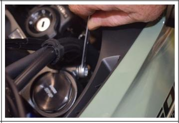
Using a 6mm Allen Key undo both lower triple pinch bolts a few turns, whilst holding the fork leg to prevent it dropping out. Slide up the fork leg about 15mm to the lower machined line of the fork tube.
