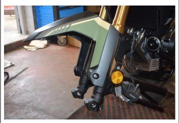
30. Remove bolt and spindle from the front wheel and insert wheel into forks, ensuring the ABS ring is facing the left fork, next to the sensor. It is preferable to remove both wheel spacers and insert some grease into the bearings before replacing the spacers, also apply a small amount of grease to the front axle to help insertion.
