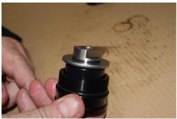
15. Ensure that the lock nut is screwed to the bottom of the threaded section before putting the new fork cap assembly on to the rod.
