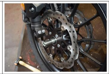
31. Slide axle through the right-hand fork leg, and through the front wheel. The when the axle is fully inserted secure with bolt from opposite side, tighten fully using 14mm hex bit on right axle end and 19mm spanner on left end.
