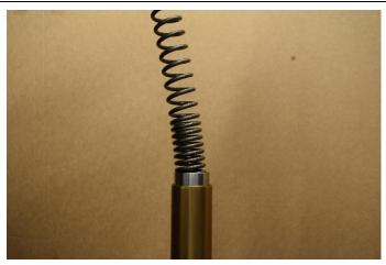
21. Fit the new Rally Raid spring, followed by the 3mm steel washer, then insert the new Rally Raid top out assembly, one person pushing down to compress the fork spring, the second person pushing down on the steel ring, and re-inserting the oem clip. Push fork cap up and down to check wire clip is seated correctly.
