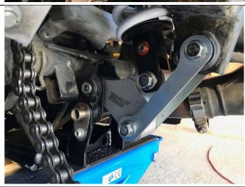
12. Attach lower shock mount to the new link (with new shorter bush fitted). Using the OEM M10 bolt and nut, but with the short spacers provided, one either side of the lower shock mount. Tighten to 40nm.
