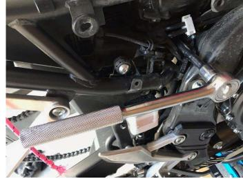
6. Using a long drift, or screwdriver, push out M10x48mm top bolt, whilst supporting shock body. Gently lower shock out of frame.
