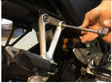
11. Fit new lower link and insert front M10x58mm bolt, tighten M10 nut (no washer) to 40Nm, using 8mm Allen key and 17mm socket.
