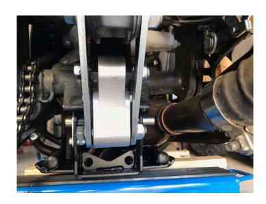
4. Undo 17mm nut on shock lower mount and remove M10 bolt. Allow OEM billet suspension link to drop down and undo 17mm nut from M10x58mm bolt securing link to frame, use 8mm Allen key to hold head of bolt. Remove bolt and remove two steel bushes from the OEM link to re-use in new link, discard the third bush. Insert both OEM steel bushes into new link, with grease and insert the new shorter bush into the new billet link where the suspension attaches, at its narrowest point.
