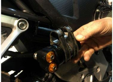
14. Position reservoir as shown and tighten hose clamp. Check reservoir body does not foul footrest hanger or brake hoses. Replace rear brake reservoir into position with original M6 bolt.
