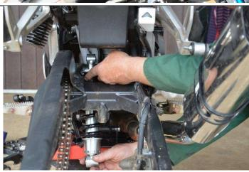
7. Insert new shock up through gap between swinging arm brace and rear of engine, with the shock positioned as shown, with the hose outlet at the 2 'O' Clock position (when viewed from rear of bike facing forward)
