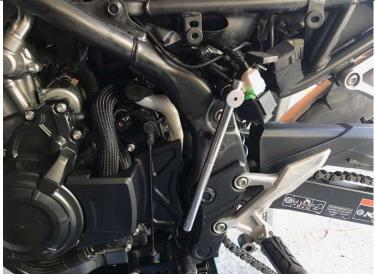
10. Remove both M8 screws holding right hand passenger footrest hanger, using 8mm Allen key. Slide in new reservoir mount between footrest hanger and frame and reinsert both M8 screws. (using Loctite or similar) Tighten to 26Nm.
